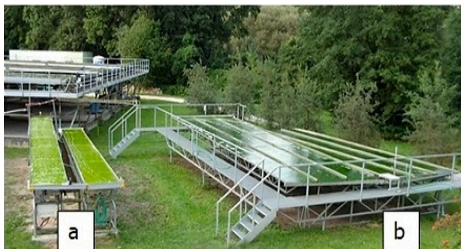
Fig. 1. (a) Outdoor thin-layer cascade of 24 m 2 was inoculated with the heterotrophically grown Chlorella g120 and (b) thin-layer cascade of 90 m 2 was used to grow the phototrophic strain of Chlorella R-117.
